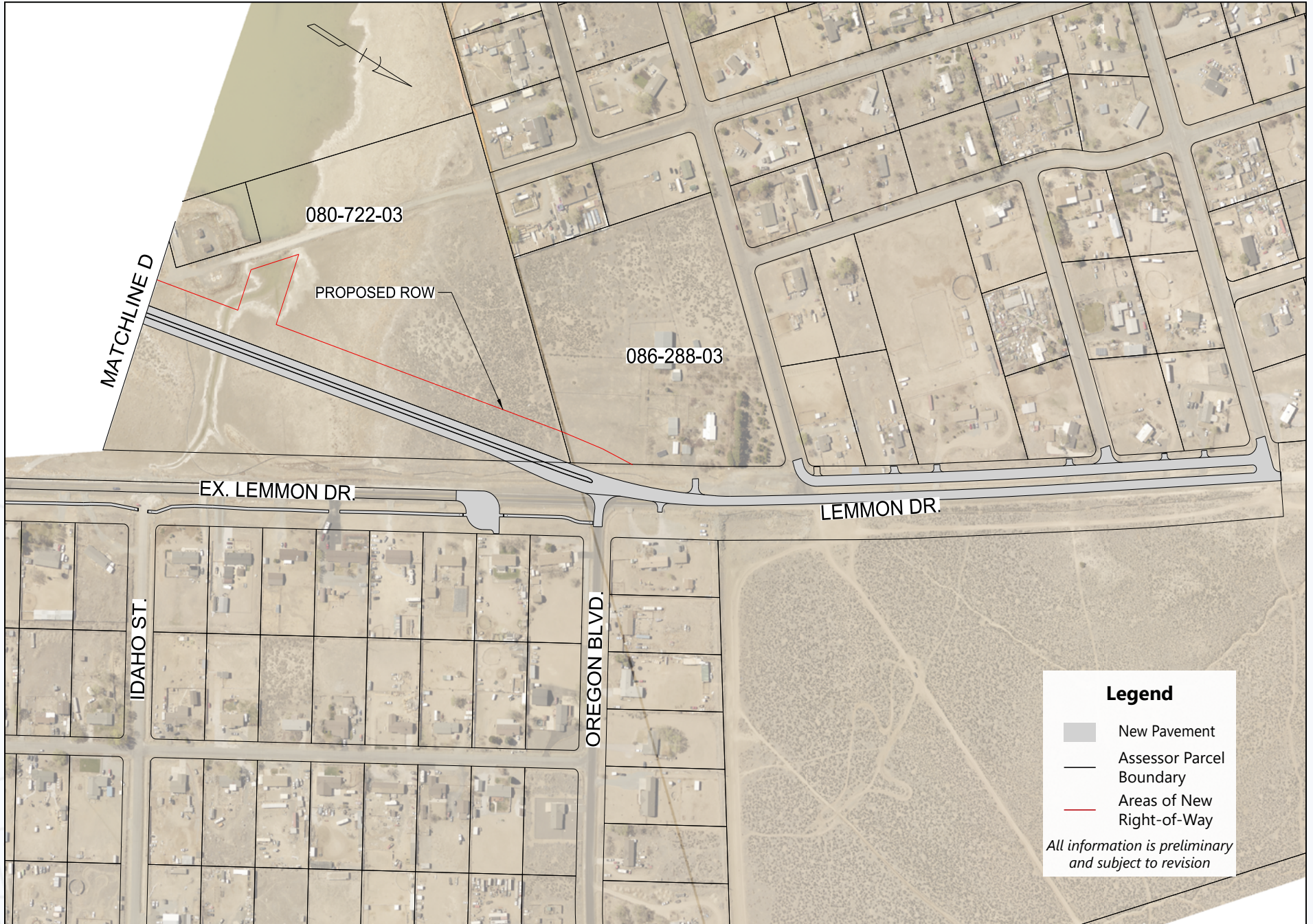
Figure 8. Areas of New Right-of-Way
